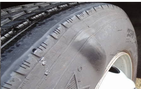
Bulge / blister — belts broken, should be replaced
