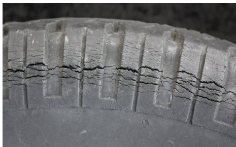
Dry rot / sidewall cracking — should be replaced
